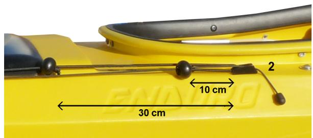
Fitting (2) for lifter line is bolted through the deck of the kayak in a suitable position beside the cockpit.
