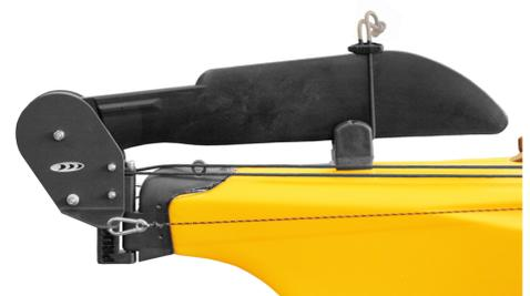
With pulling the rear ball to front the blade can now be moved from the water to the deck or the other way. With the fixing line the blade can be secured from sliding up during paddling. On deck the V-shaped blade support provides a fixed position for the blade and includes a transport fixing.
